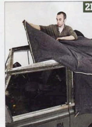
...and then lift it up and into place on the hood sticks.
