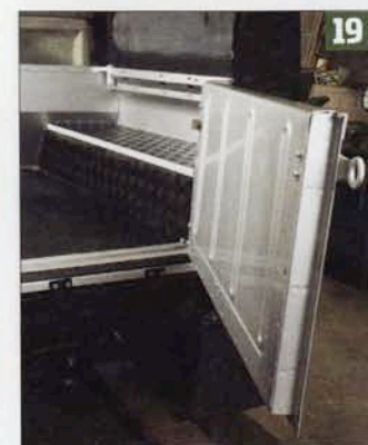
Another option is to re-use the rear door hinges and catch, and create your own side-hinged rear tailgate.
