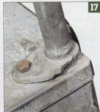
The hoops are held in place on the body cappings by these clips; if these (or the rear fixings) are missing, you can get them from Exmoor Trim.
