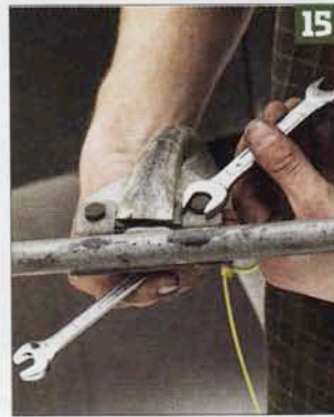
The centre support can now be bolted to the side bars - make sure you get it the right way around to avoid snagging on the canvas.
