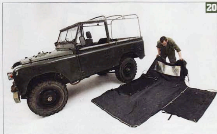
If the canvas hasn't been folded for easy fitting, lay it flat alongside the vehicle...
