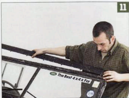
First to go on is the screen rail. There are slight differences between Series I and later leaf-sprung Land Rovers, and Defenders use a totally different arrangement that 'grips' the front of the canvas. It's held in place using the existing bolt holes. Leave the end pairs empty for the moment.
