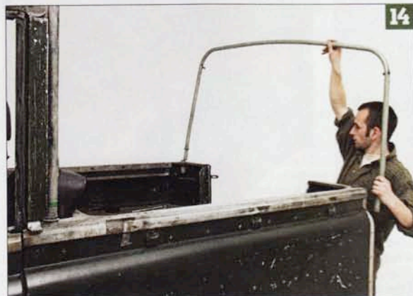
The rear hoop can now be lifted into place. On a long-wheelbase 110 or 109 there's a central hoop to slot in as well.
