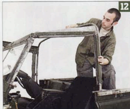
The front hoop can now be dropped into place in the large holes previously occupied by the roof corner bolts. If your set comes fully dismantled, it's a simple job to attach the door surrounds.
