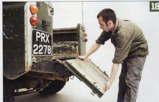
The tailgate can now be fitted; it simply slides into the brackets on the rear crossmember. If your Defender is missing them, you can get them as part numbers MUC8738 and MUC8739. If the tailgate doesn't want to close, you'll find some adjustment by slackening off the hinge bolts.
