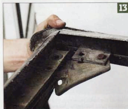
The door top surrounds slot into the windscreen rail and are joined by this triangular plate. With bolts through the windscreen, the rail and the plate, the corners are now secure.
